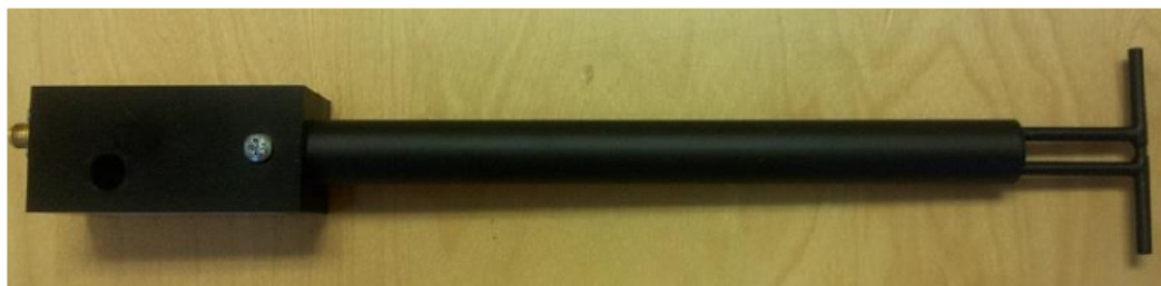
Figure 1 – MVG COMOSAR Validation Dipole
