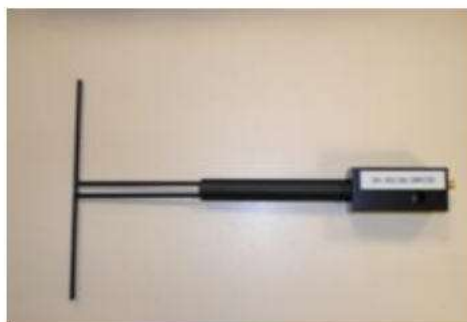
Figure 1 – Satimo COMOSAR Validation Dipole
