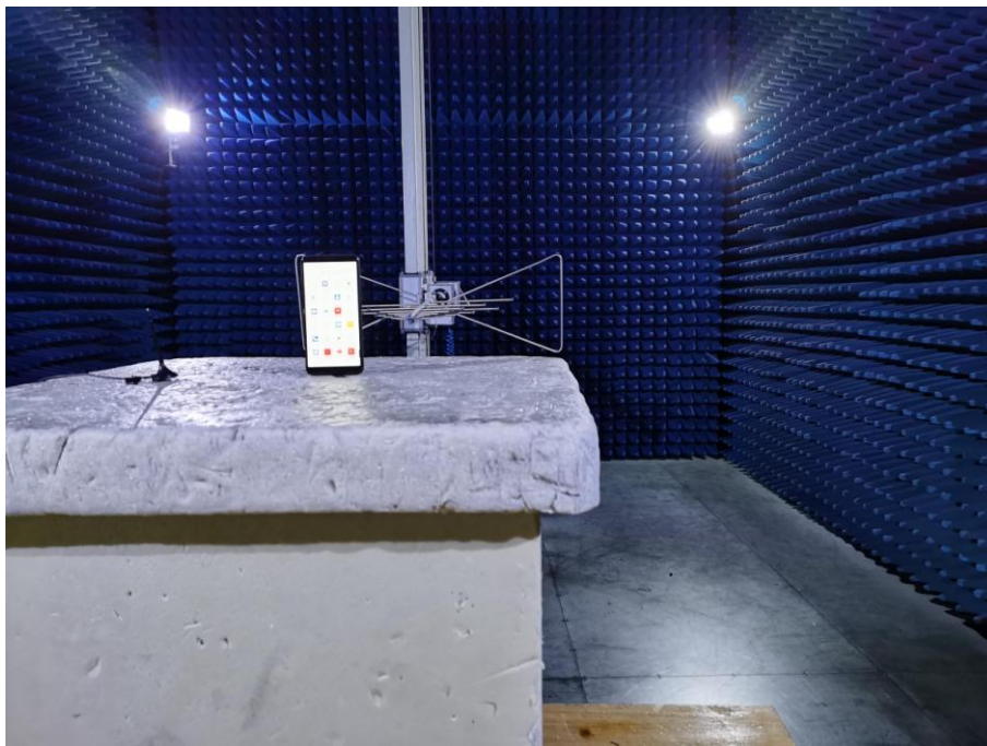
Radiated Spurious Emissions Test View (Above 1GHz)
