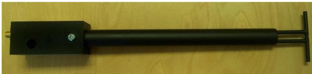
Figure 1 – MVG COMOSAR Validation Dipole
