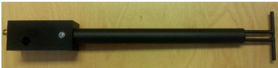
Figure 1 – MVG COMOSAR Validation Dipole
