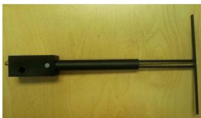
Figure 1 – MVG COMOSAR Validation Dipole
