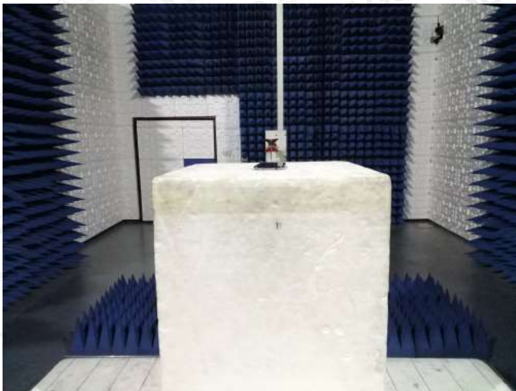
RADIATED SPURIOUS EMISSION-ABOVE 1G TEST SETUP
