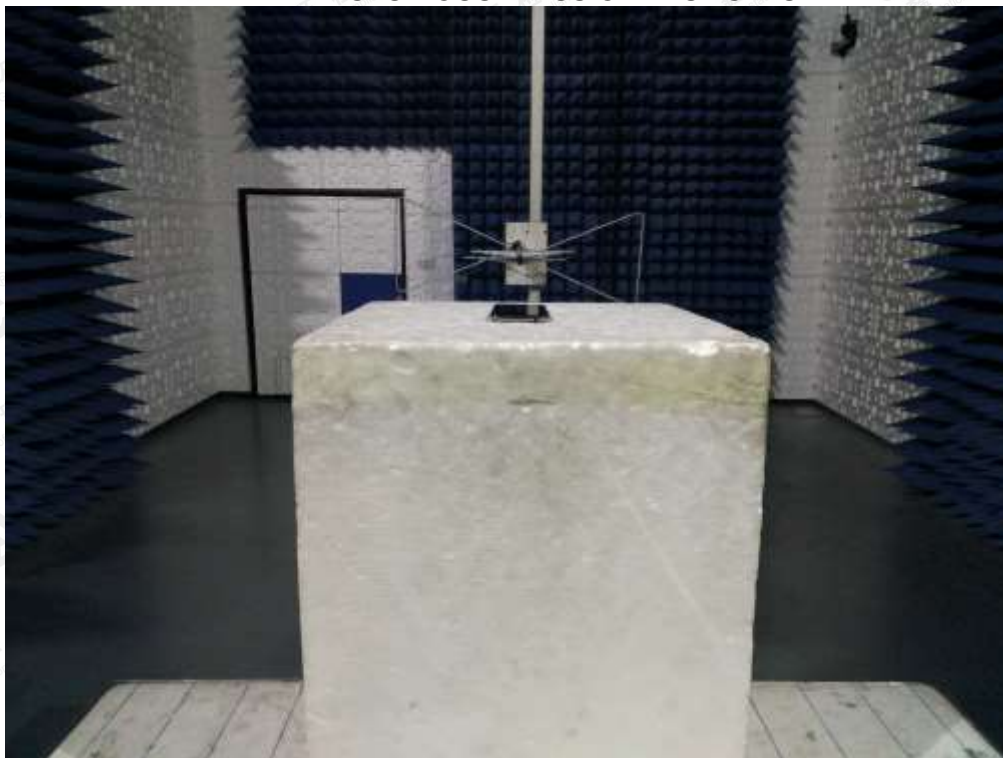
RADIATED SPURIOUS EMISSION-ABOVE 1G TEST SETUP
