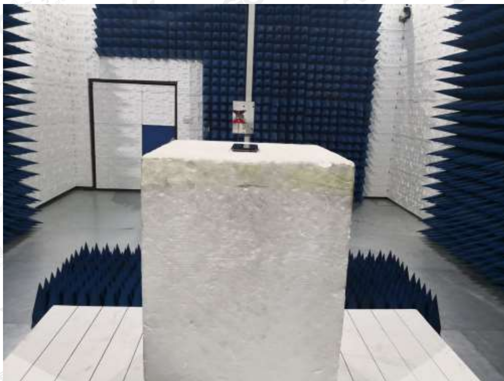
RADIATED SPURIOUS EMISSION ABOVE 1G TEST SETUP
