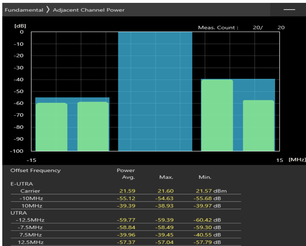
Band7 QPSK BW=10MHz Channel=21100 RB Size=50 Position=#0
