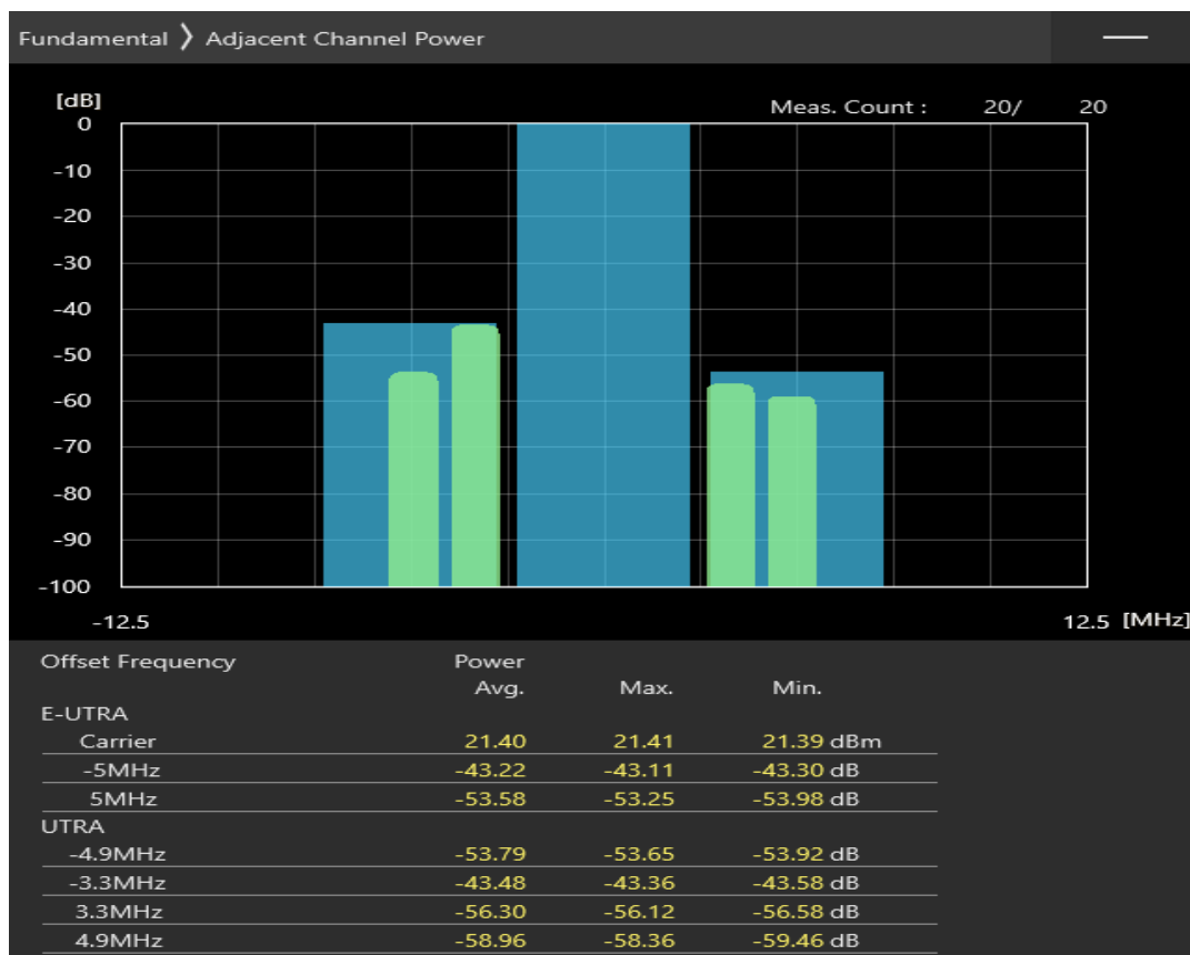
Band41a QPSK BW=5MHz Channel=40740 RB Size=8 Position=#Max
