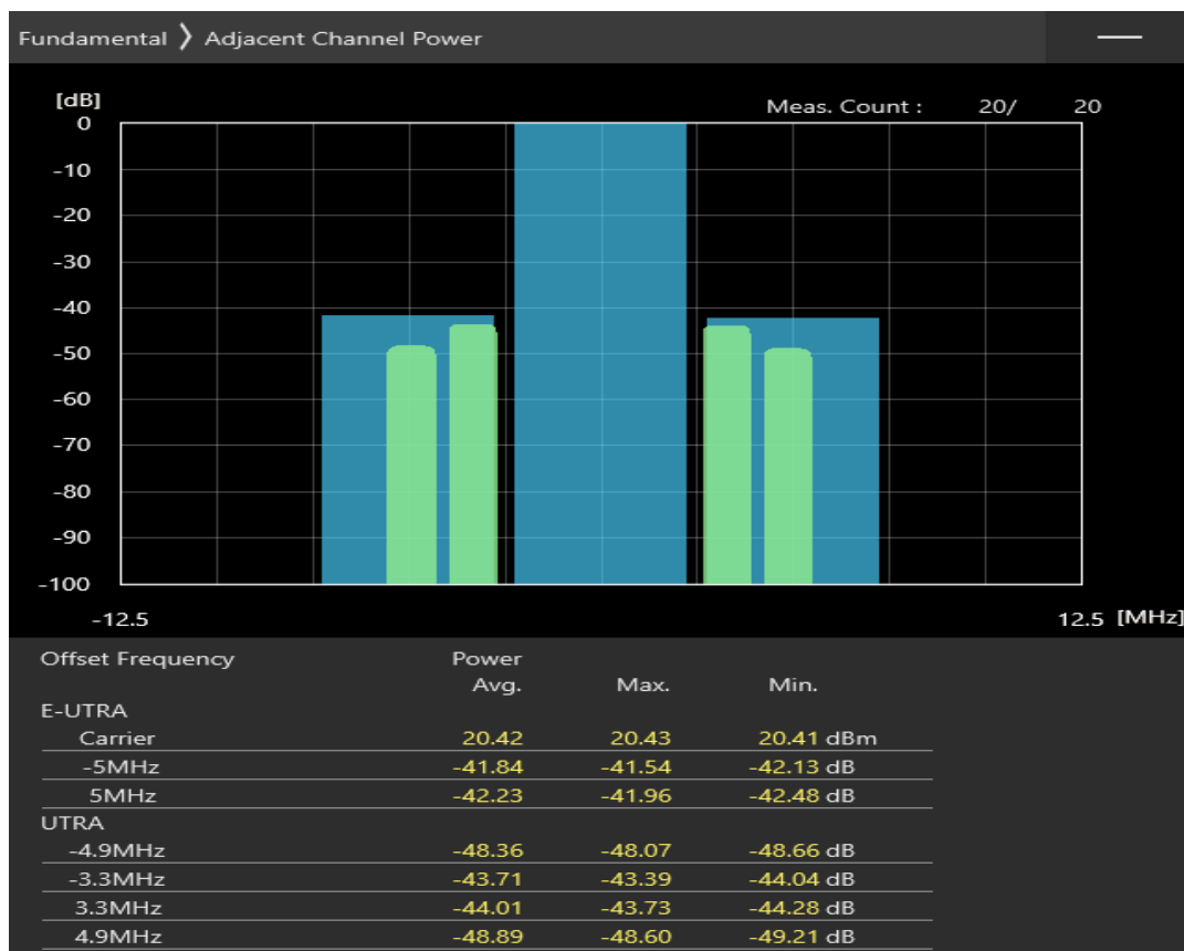
Band41a 16QAM BW=5MHz Channel=40740 RB Size=8 Position=#0
