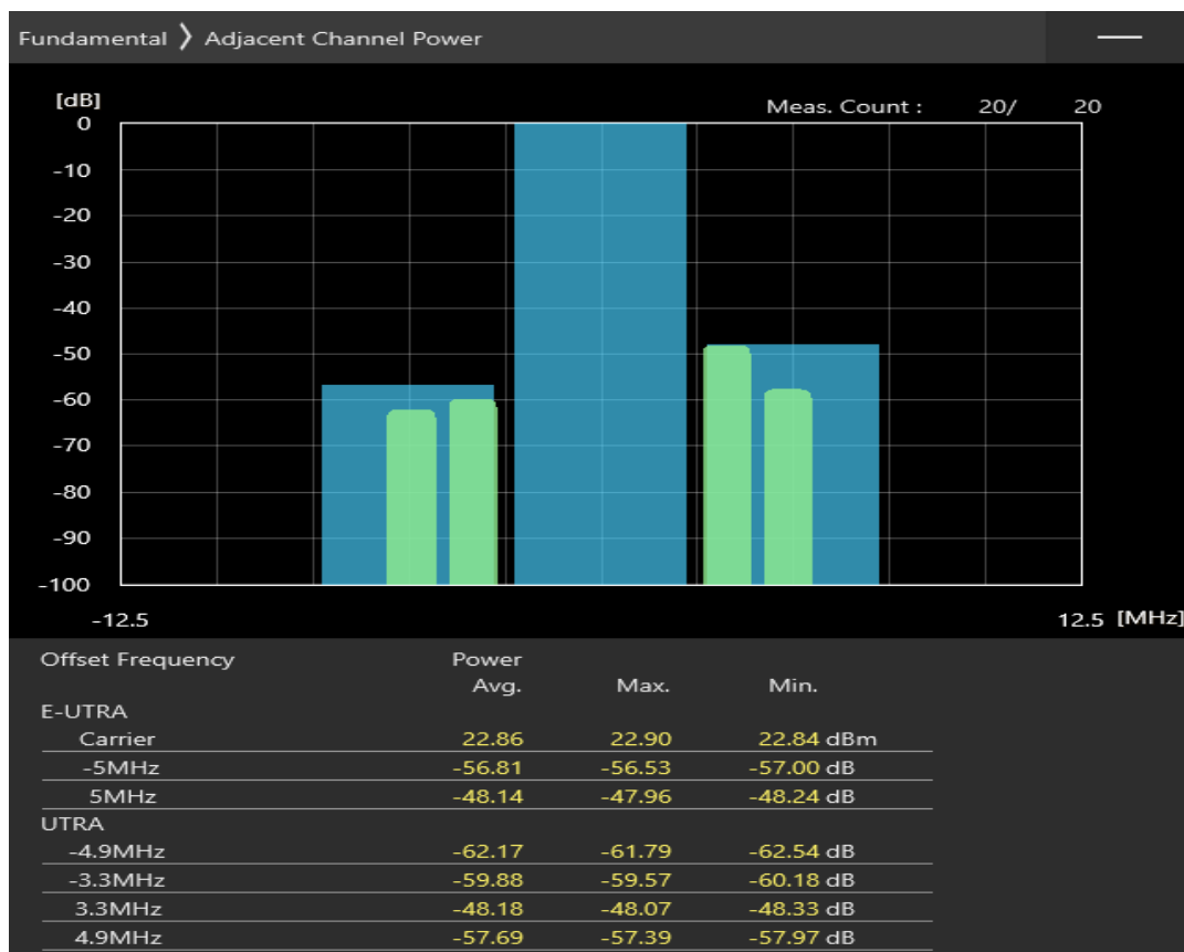
Band40 QPSK BW=5MHz Channel=39625 RB Size=25 Position=#0
