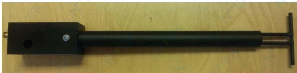
Figure 1 – MVG COMOSAR Validation Dipole
