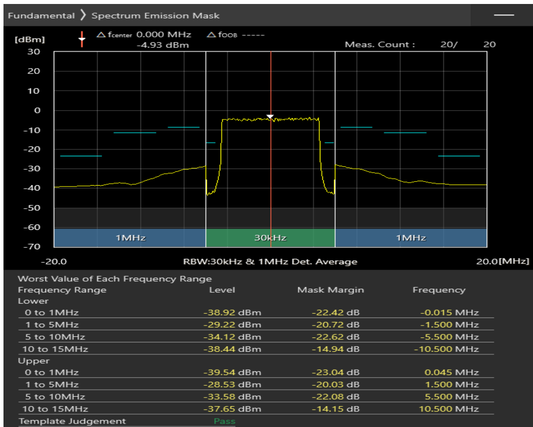
Band41a 16QAM BW=10MHz Channel=40090 RB Size=12 Position=#0
