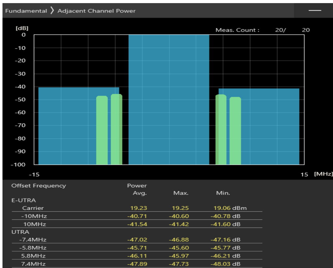
Band41a QPSK BW=10MHz Channel=41190 RB Size=12 Position=#0
