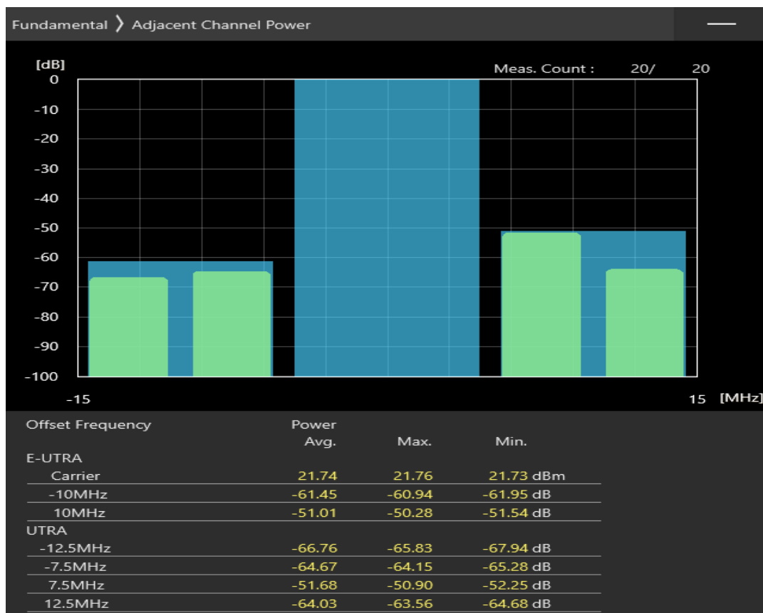
Band3 QPSK BW=10MHz Channel=19250 RB Size=50 Position=#0
