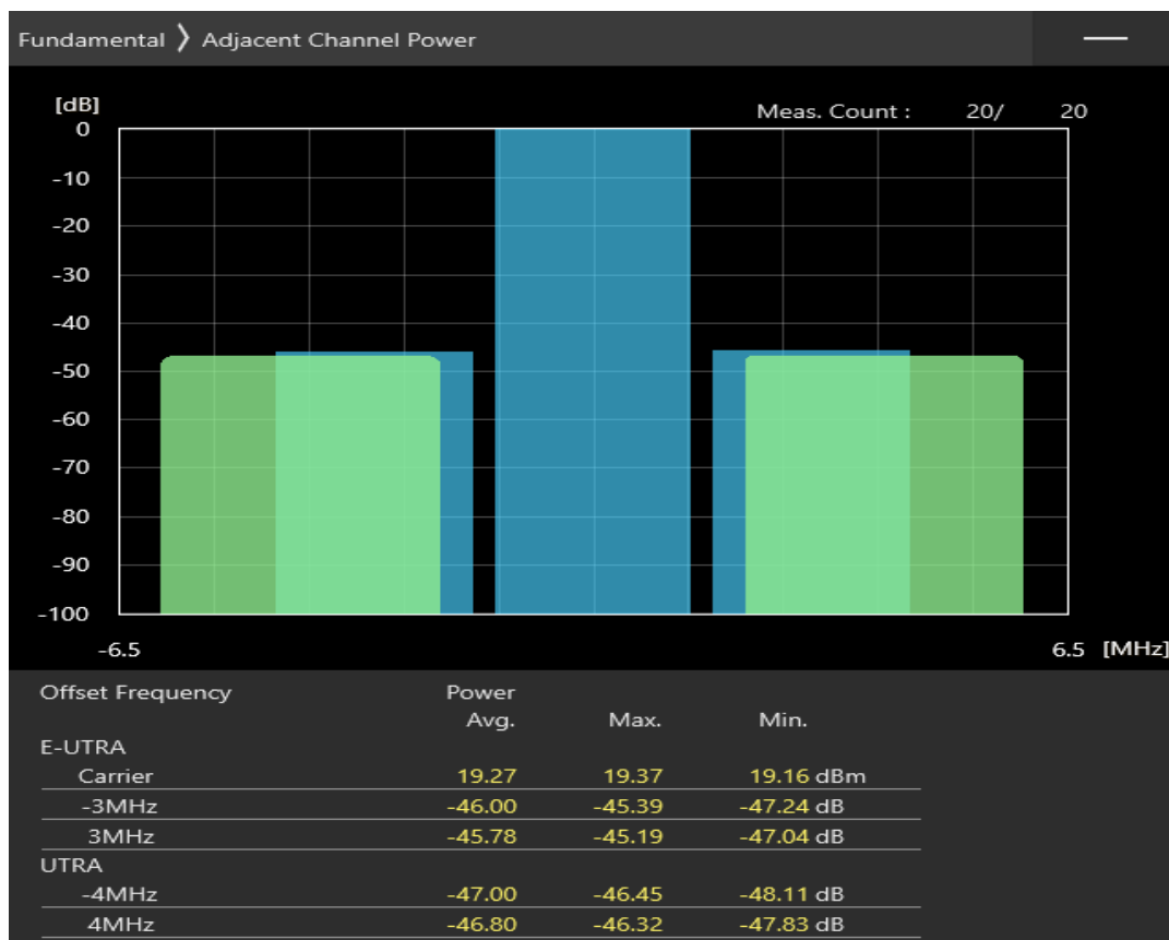
Band28 QPSK BW=5MHz Channel=27235 RB Size=8 Position=#0
