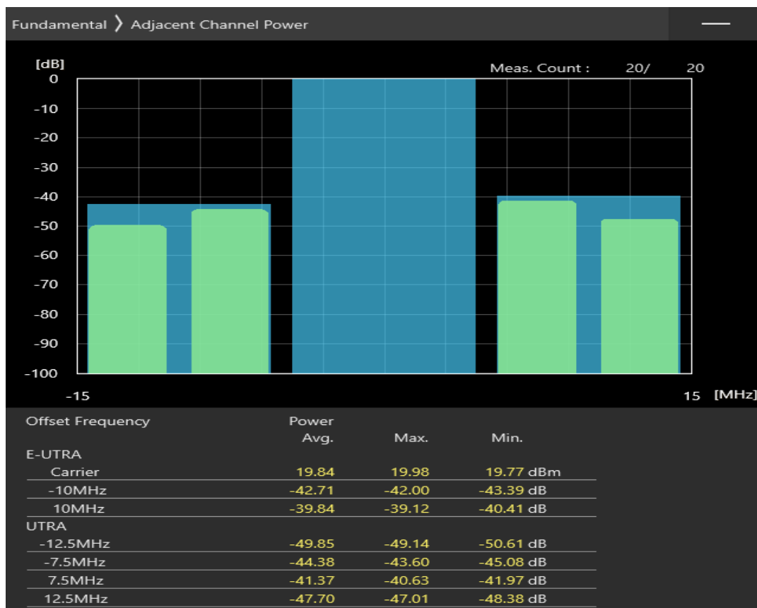
Band7 QPSK BW=10MHz Channel=21400 RB Size=12 Position=#0
