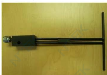
Figure 1 – MVG COMOSAR Validation Dipole
