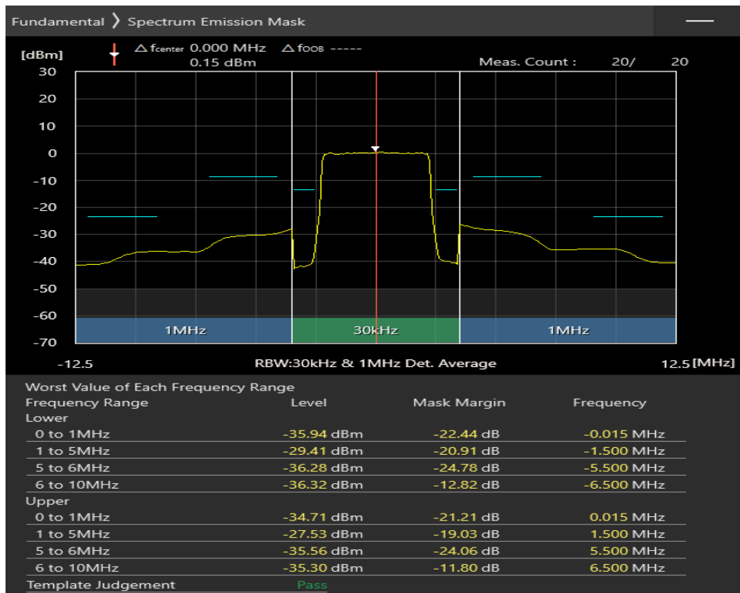
Band1 16QAM BW=5MHz Channel=18025 RB Size=8 Position=#0
