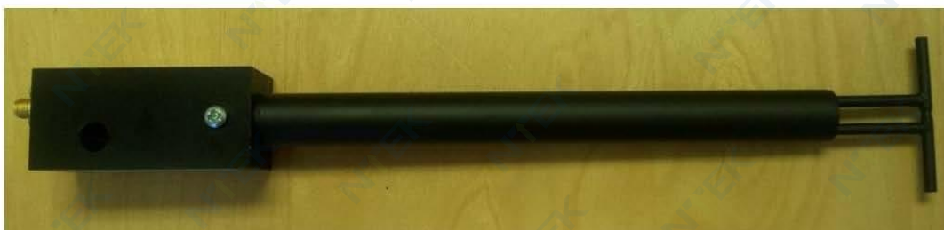
Figure 1 – MVG COMOSAR Validation Dipole
