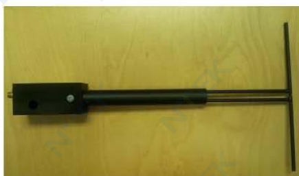
Figure 1 – MVG COMOSAR Validation Dipole
