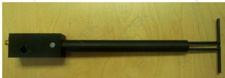
Figure 1 – MVG COMOSAR Validation Dipole
