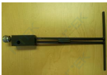
Figure 1 – MVG COMOSAR Validation Dipole
