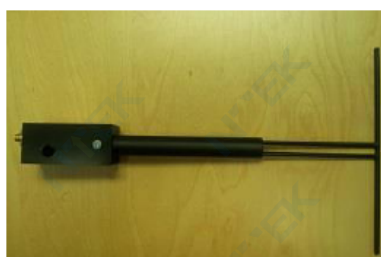
Figure 1 – MVG COMOSAR Validation Dipole
