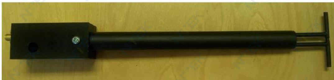
Figure 1 – MVG COMOSAR Validation Dipole
