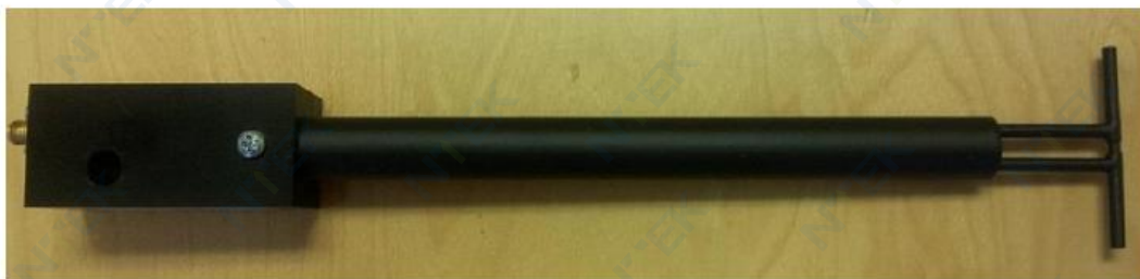
Figure 1 – MVG COMOSAR Validation Dipole
