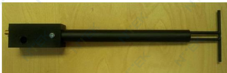
Figure 1 – MVG COMOSAR Validation Dipole
