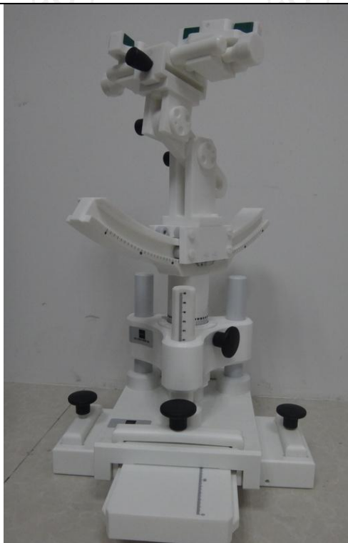
COMOSAR Mobile phone positioning system
