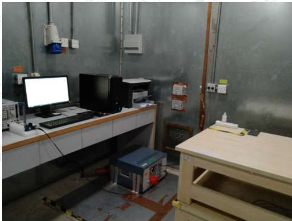
RADIATED EMISSION TEST SETUP
