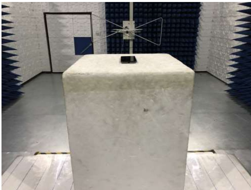
RADIATED SPURIOUS EMISSION-ABOVE 1G TEST SETUP
