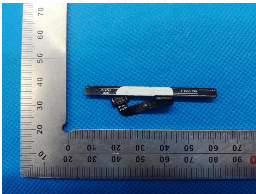
Fig.12 – bottom circuit of battery
