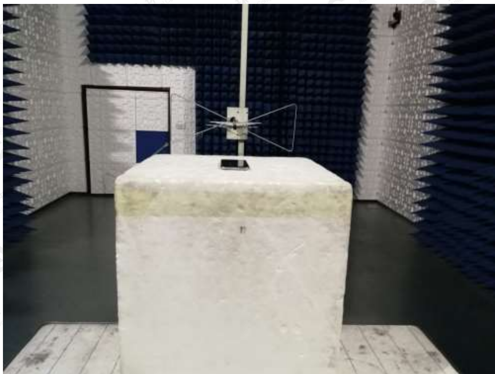
RADIATED SPURIOUS EMISSION-ABOVE 1G TEST SETUP
